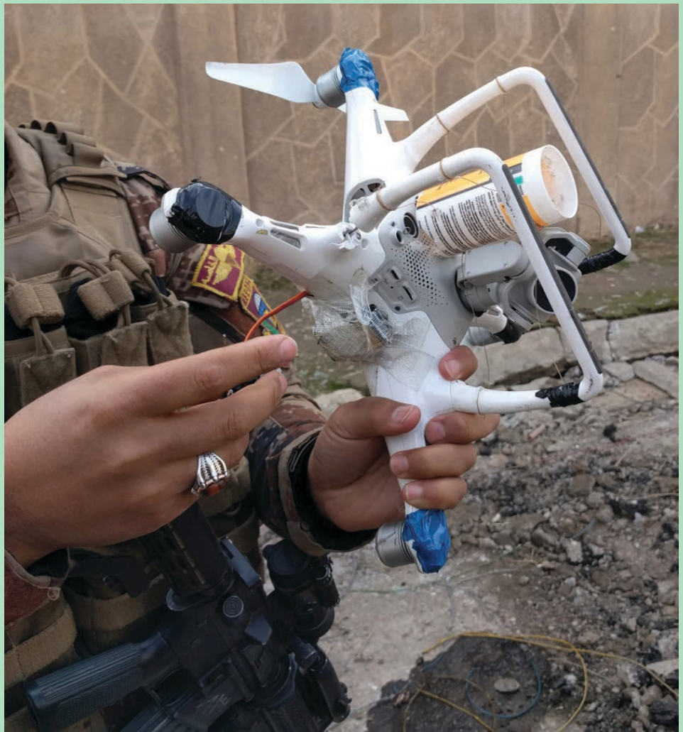
An allied Soldier displays a Group 1 UAS quadcopter modified for the deployment of a 40 mm grenade. (Michael Utterback/Courtesy photo)
