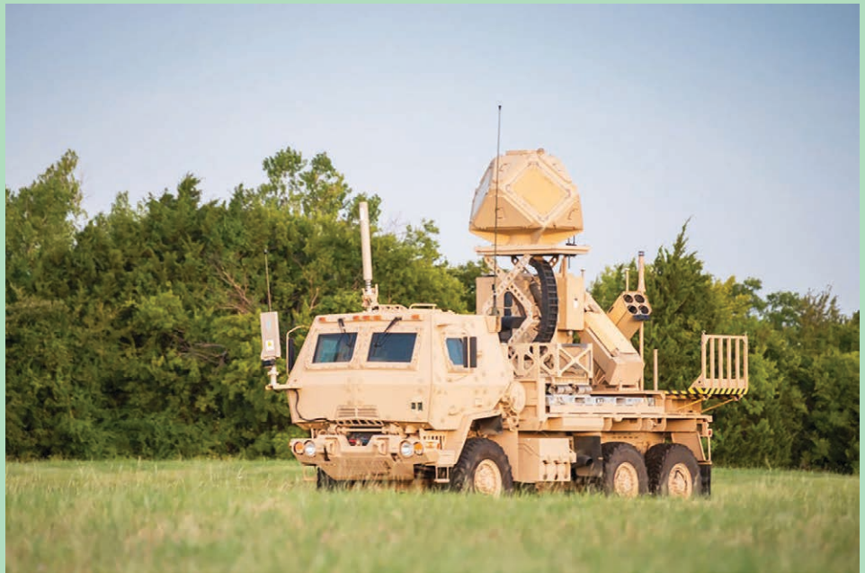
A Howler system with a KuFRS Radar and Coyote CUAS launchers. The Howler uses the Coyote missile which is a missile-like drone to destroy threats not engageable by the LPWS. (Photo courtesy Raytheon)
