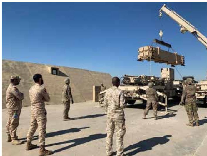
The 3-2nd ADA BN and Kuwaiti Soldiers conduct reload operations on a PAC-3 Launcher.
