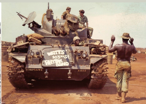
The M42 40 mm Self-Propelled Anti-Aircraft Gun, or “Duster,” is an American armored light air-defense gun built for the United States Army from 1952 until December 1959, in service until 1988. (Photo credits: Left, Mark Pellegrini, U.S. Army Ordnance Museum [Aberdeen Proving Ground, MD] Creative Commons CC-BY-SA-2.5; Middle: the Army Historical Foundation; Right: Bill Maloney, Pennsylvania Military Museum)
