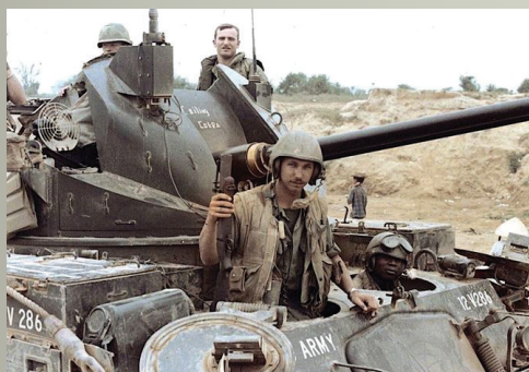
The M42 40 mm Self-Propelled Anti-Aircraft Gun, or “Duster,” is an American armored light air-defense gun built for the United States Army from 1952 until December 1959, in service until 1988. (Photo credits: Left, Mark Pellegrini, U.S. Army Ordnance Museum [Aberdeen Proving Ground, MD] Creative Commons CC-BY-SA-2.5; Middle: the Army Historical Foundation; Right: Bill Maloney, Pennsylvania Military Museum)
