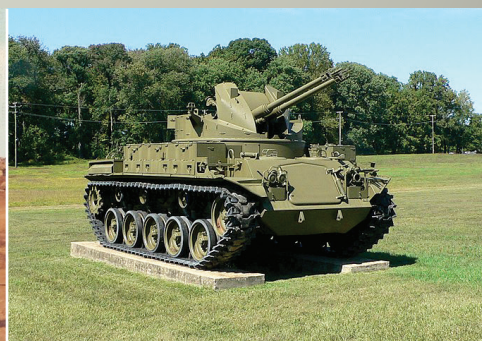
The M42 40 mm Self-Propelled Anti-Aircraft Gun, or “Duster,” is an American armored light air-defense gun built for the United States Army from 1952 until December 1959, in service until 1988. (Photo credits: Left, Mark Pellegrini, U.S. Army Ordnance Museum [Aberdeen Proving Ground, MD] Creative Commons CC-BY-SA-2.5; Middle: the Army Historical Foundation; Right: Bill Maloney, Pennsylvania Military Museum)
