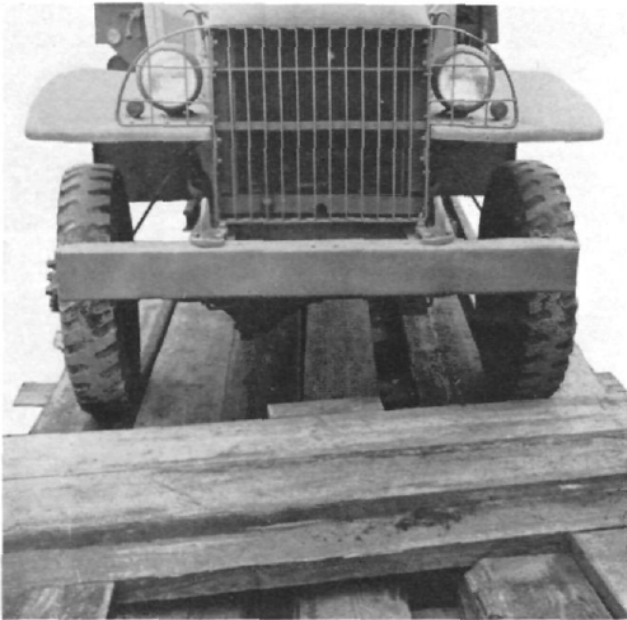
Fig. 6—The rails won't tear the wheels off your trucks if you pave 'em with lumber.
