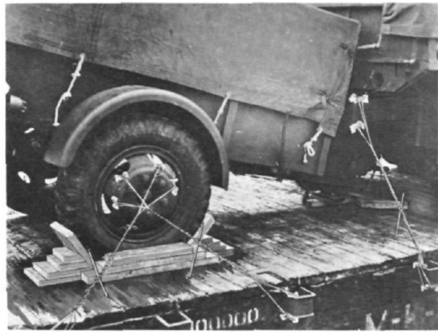
Fig. 11—Tighten the wire with the drift pin—then sink the pin into the floor.
