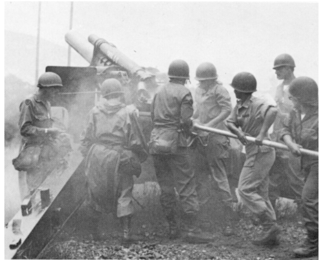
An all-female team rams a 155-mm round into the M114A1 howitzer as trained male artillery safety inspectors watch during HEL tests. (Photo by Gene Bonhage)
