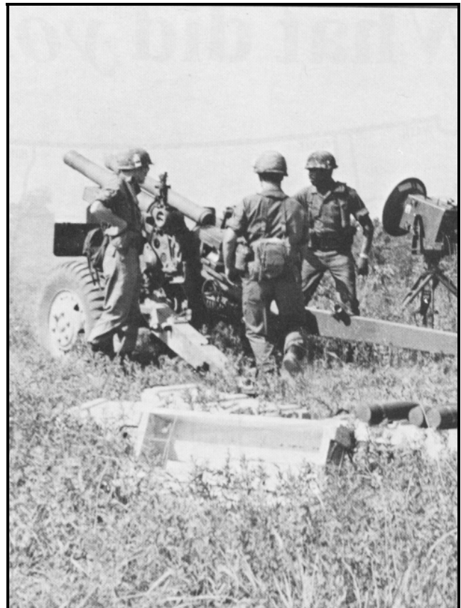
C Battery, 1-36th FA (Ohio ARNG), measures the muzzle velocity of its howitzers with chronographs operated by the 101st Airborne Div Arty at Fort Campbell. (Photo by Lee Hunter)
