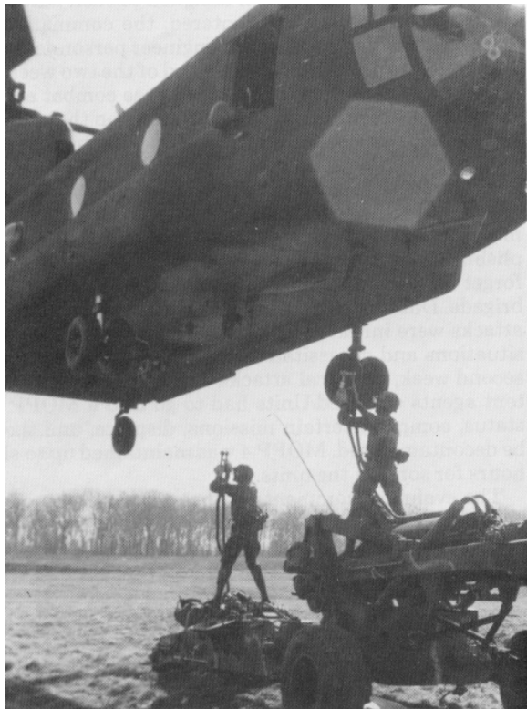
FORT CAMPBELL, KY —Soldiers from the 2d Battalion, 31st Field Artillery, 101st Airborne Division (Air Assault), complete the final hook-up of an M198 155-mm howitzer for a practice raid across the forward edge of the battle area at Fort Campbell, Kentucky. (Photo by PFC Bill Powell)
