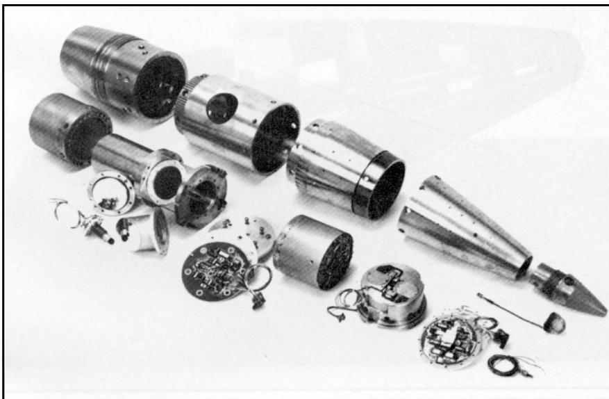
Figure 2: VIP consists of a 155-mm projectile body and the mechanical, optical and electronic sub-assemblies necessary to collect video images of the terrain over which the projectile flies.
