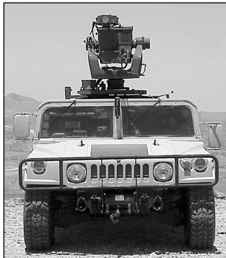
The fire support sensor system (FS 3 ) will be mounted on the Knight vehicle in 2005.
