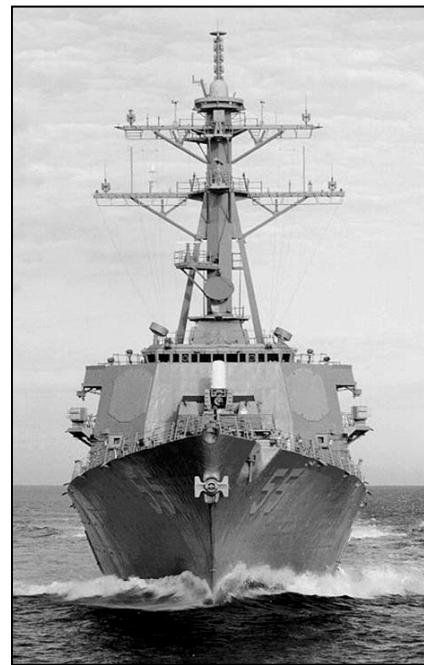
An Arleigh Burke-Class Guided-Missile Destroyer, DDG 55 USS Stout with SPY-1D Metal Plates
