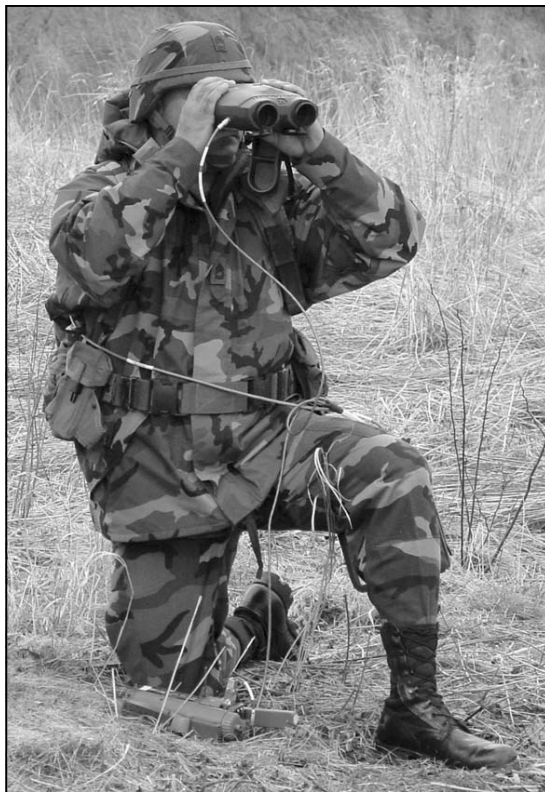
A soldier using the Leica Viper/Vector 21 wired to the PFED. (Photo by Jeffrey Weiss)
