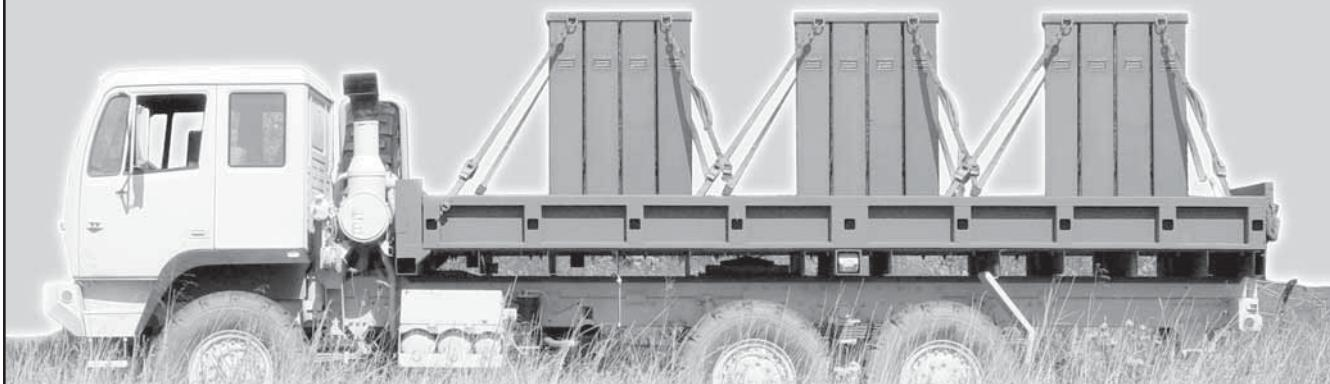
NLOS-LS Flexibility and Capability. As shown in the photo, three container launcher unit (CLU) mockups are carried on the bed of a family of medium tactical vehicles.
