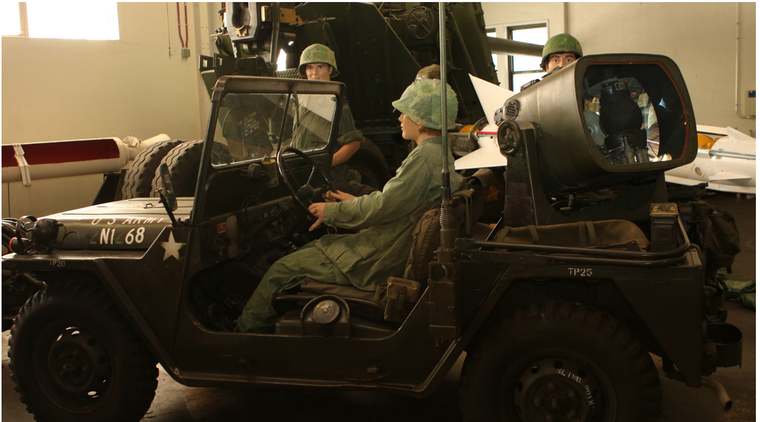
Above: ADA – The GS14, a 23-inch xenon searchlight, were simple and effective to use and were small enough to fit on a standard M-151 jeep. The lighter lamps only put out 120 million candlepower.
