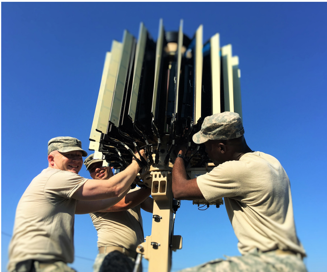
From the left, Chief Warrant Officer 2 Chris Fortune, Spec. Mike Stevenson and Warrant Officer Candidate Armand Hunter assemble the AN/TPQ-50 Lightweight Counter-Mortar Radar system, July 23, 2016, as part of annual training with the 1st Battalion, 101st Field Artillery Regiment, at Joint Base McGuire-Dix-Lakehurst. (Staff Sgt. Steven Littlefield/1st BN, 101st FA)
