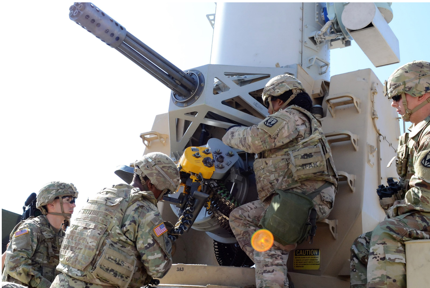
Soldiers from the 5th Battalion, 5th Air Defense Artillery, perform maintenance checks on a Land-based Phalanx Weapons System during the battalion's pre-deployment mission readiness exercise at Fort Sill, Okla., in August 2016. (Staff Sgt. Mark Kauffman/U.S. Army)
