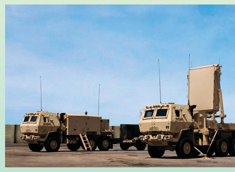
The AN/TPQ-53 system (shown here in its fully upgraded configuration) is the Army's next-generation counter-fire target acquisition radar. It is scheduled to replace the EQ-36 QRC in 2019. (Paul Salce/Lockheed Martin Corp.)
