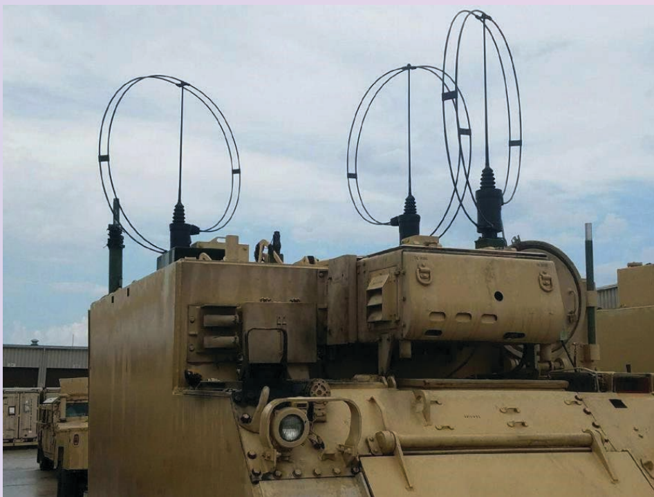
The near vertical incident skywave loop antennae installed on M1068 Battalion Fire Direction Center. (Courtesy photo)
