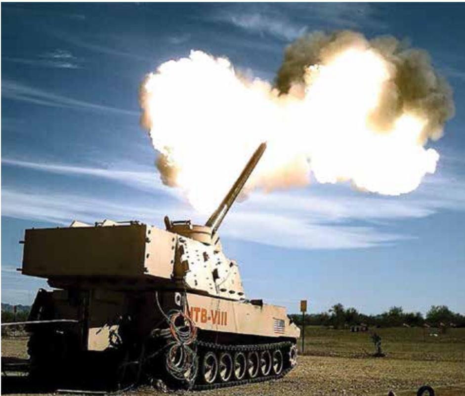
Extended Range Cannon Artillery, or ERCA, will be an improvement to the latest version of the Paladin self-propelled howitzer that provides indirect fires for the brigade combat team and division-level fight. Building on mobility upgrades, ERCA will increase the lethality of self-propelled howitzers. ERCA provides a “10x” capability through a combination of an increased range, increased rate of fire, increased lethality, increased reliability and a greater survivability. Photo by Edward Lopez, June 12, 2018
